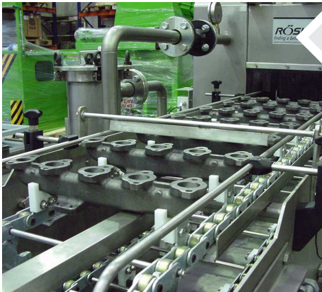
Transport with V supports for washing and drying.
