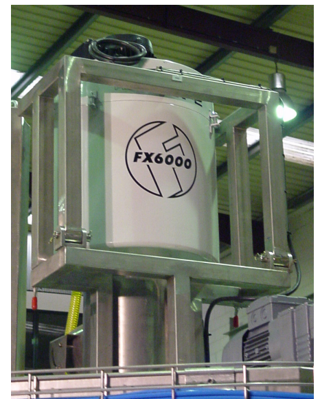
Vapor aspiration system using centrifuge condenser
